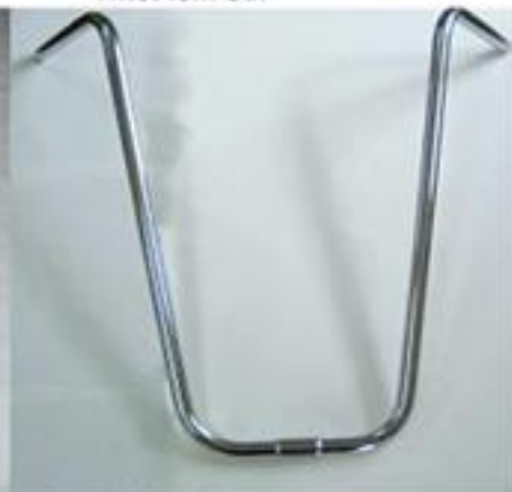
CH-HD04 CP For recumbent W/660 x R/470,530,635 x Ø25.4
