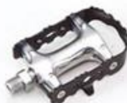
CH-734B Body: Die casting alloy body with steel cage. Spindle: CNC machined CrMo Bearing: sealed / DU bushing
