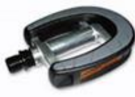
CH-744B Body: Die casting alloy body with non-slip cage Spindle: CNC machined CrMo Bearing: sealed / DU bushing
