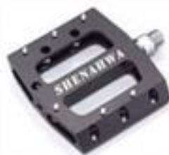
CH-011 Body: aluminum 6061 extruded CNC Machined wireplaceable pins Spindle: CNC machined Cr-Mo Bearing: sealed / DU bushing
