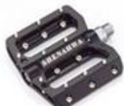
CH-700B Body: Die casting alloy body Spindle: CNC machined CrMo Bearing: sealed / DU bushing Pins: Replaceable pins.
