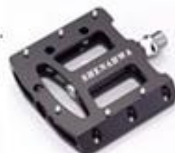
CH-010 Body: aluminum 6061 extruded CNC Machined wireplaceable pins Spindle: CNC machined Cr-Mo Bearing: sealed/DU bushing
