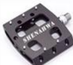
CH-013 Body: aluminum 6061 extruded CNC Machined wireplaceable pins Spindle: CNC machined Cr-Mo Bearing: sealed / DU bushing
