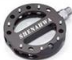
CH-014 Body: aluminum 6061 extruded CNC Machined wireplaceable pins Spindle: CNC machined Cr-Mo Bearing: sealed / DU bushing
