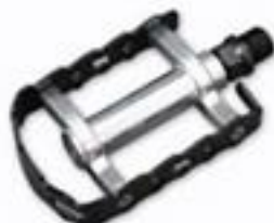
CH-743B Body: Die casting alloy body with steel cage Spindle: CNC machined CrMo Bearing: sealed / DU bushing
